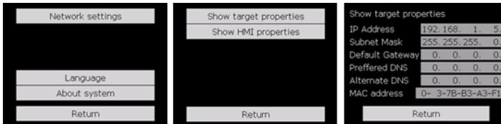
On the "Show target properties ", the required IP address of the aggregate is displayed on the first line.
