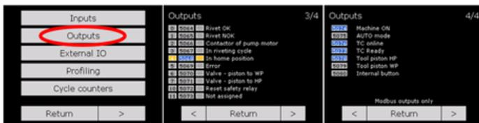
External IO screens allow the user to control individual virtual inputs and outputs (IO controlled via Modbus TCP). This is useful for parent system programming and integration testing. Switching on the forced input/output activates the virtual input/output, i.e. the bit at the address designated for Modbus TCP. Physical input/output is not affected.
