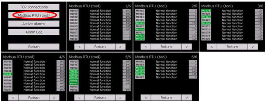
Buttons "Active alarms" and "Alarm Log" refer to the active alarm and alarm log screens shown in the Control and Monitoring chapter.
