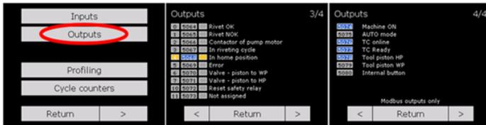
Profiling screens are used to monitor the timings of various operations performed by the system. For the user's needs, the times of the riveting operation are available for viewing. For the measured process, the times of the current cycle, average time, maximum and minimum measured time of one cycle are displayed.
